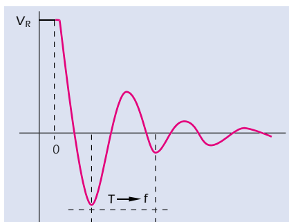
B32861...B32862: Discharge curve (ignition unit)
